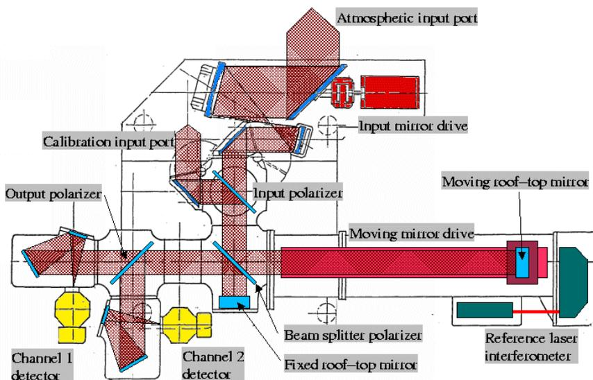
Fig. 1 - Schematic layout of the IBEX interferometer
